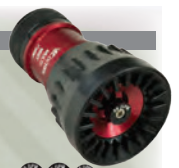
NZ028 Multi-Mist Nozzle • 1" hose connection • 4 Interchangeable tips 15, 25, 35, 55 GPM
