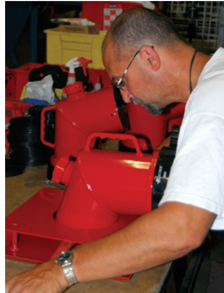
Matt Rodman assembles a low-level drafting strainer with a 6-inch, long-handle threaded coupling, signature products for Kocheck.
