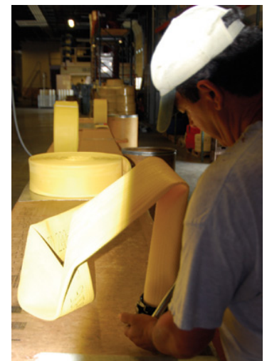
Joe Rocha installs a Storz head coupling on 4-inch large diameter hose, a relatively new product in the Kocheck catalog. (Fire Apparatus Photo)
