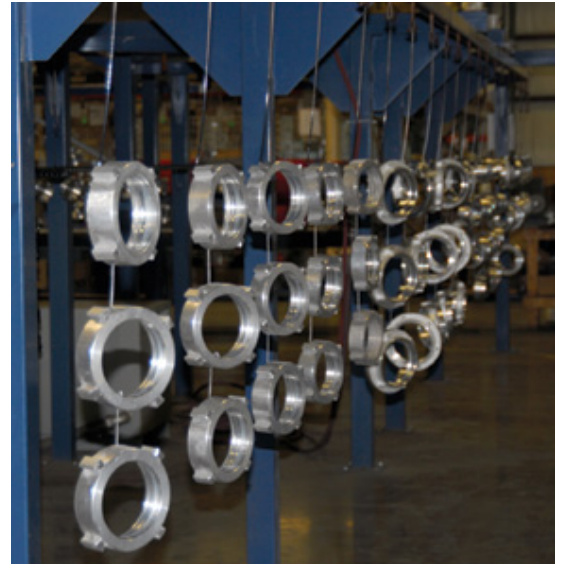
Female rocker lug 2.5-inch fittings, and other parts, are hung in rows on a conveyor system to receive a powder coat finish. Kocheck does powder coating in-house, offering a rainbow of colors.
